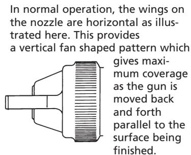
**Spray width adjustment:** Turn clockwise for round, counterclockwise for fan.
