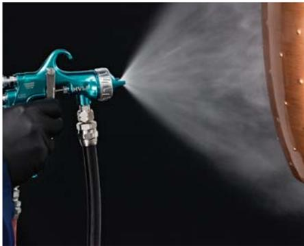
Each gun can be configured with the appropriate needle and nozzle to accommodate the coating, size of part and type of surface to be finished.
